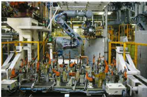
JIG & ROBOT設備 Equipment with jigs and robots 夹具和机械手的结合体设备
