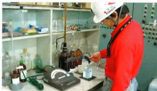
処理水のPH測定 pH measurement of processed water 处理水的PH测定
